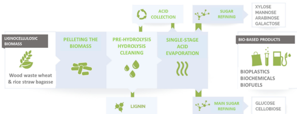
Figure 8: Production of industrially fermentable sugars from lignocellulose-containing residual biomass by Green Sugar AG
